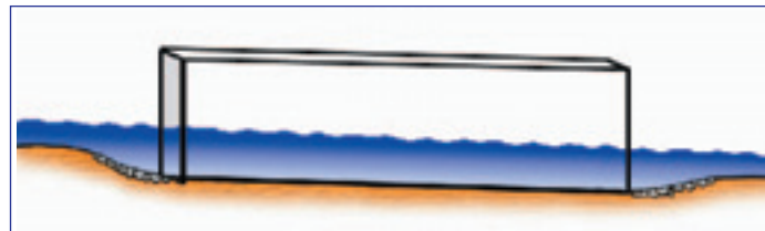
Fig. 2. Over-sized box culvert permanently backwatered
